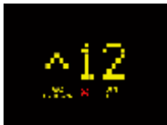
6.4" EOD-LCD Yellow dot matrix liquid crystal display
